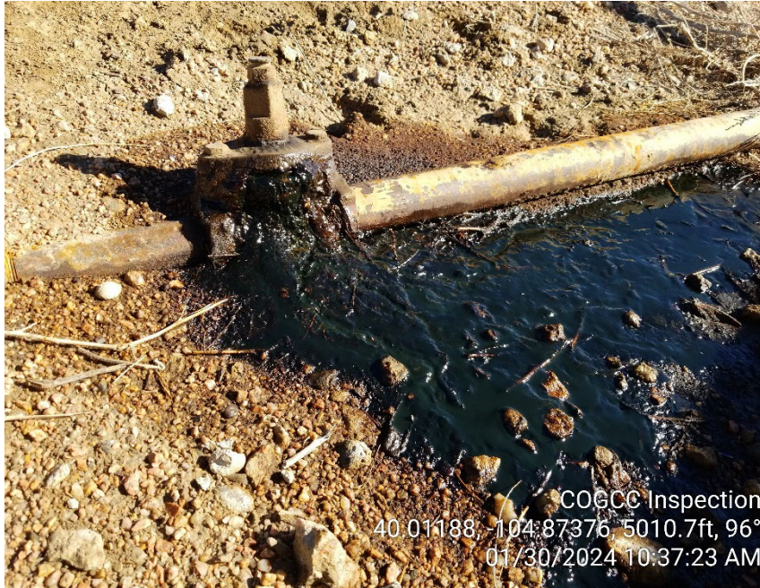
Photo 5 – Leak at separator
