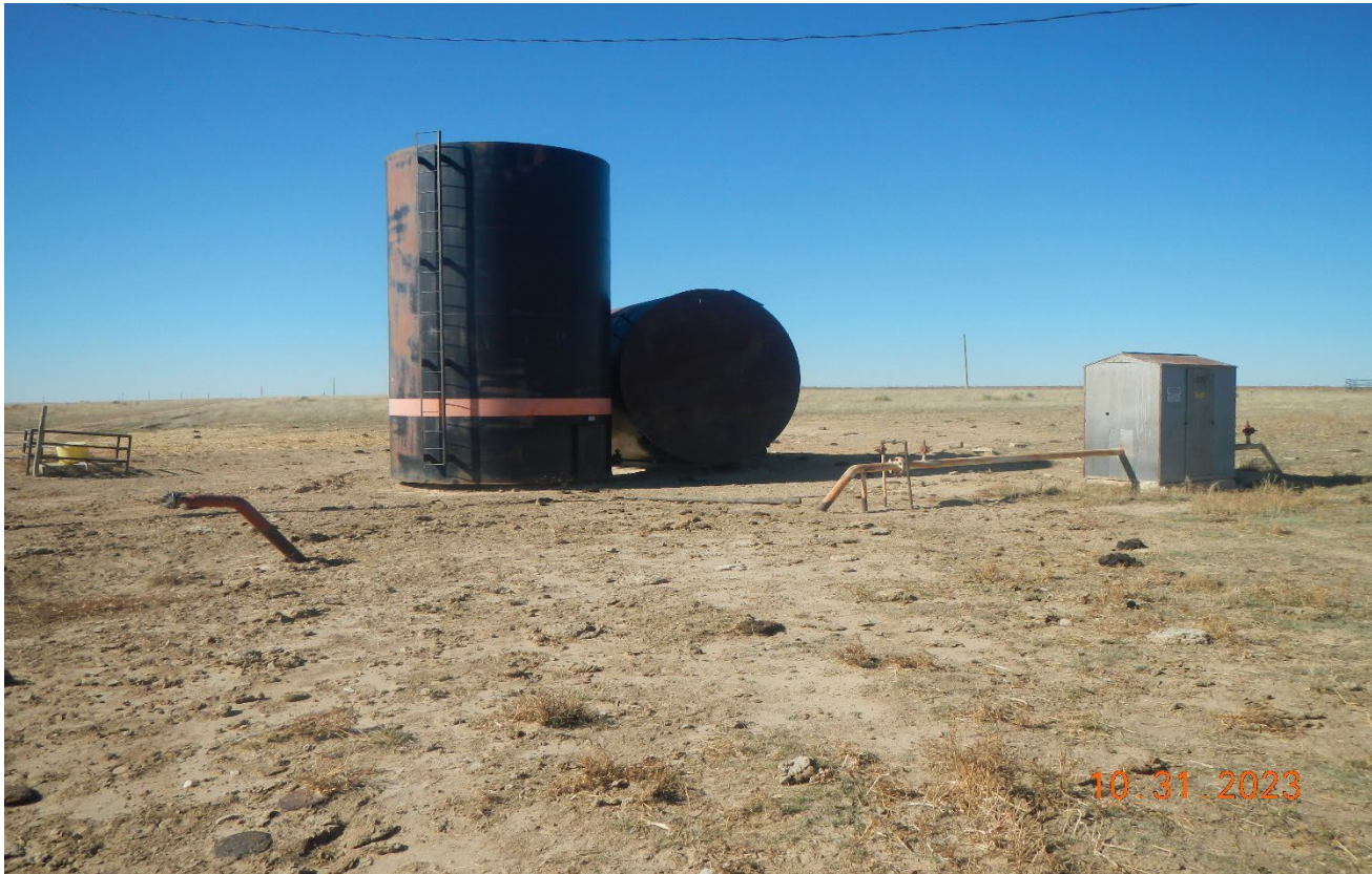
Photo 3. There are two tanks, pipe riser, meter run, and cement debris that remain. All equipment should have been removed within 3 months of well abandonment.
