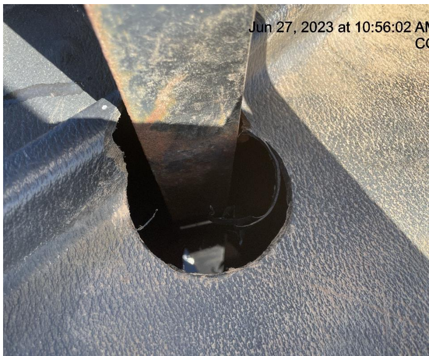
Photo # 2060 Chemical containment approximately 5/8 full - Failure to maintain chemical BMP
