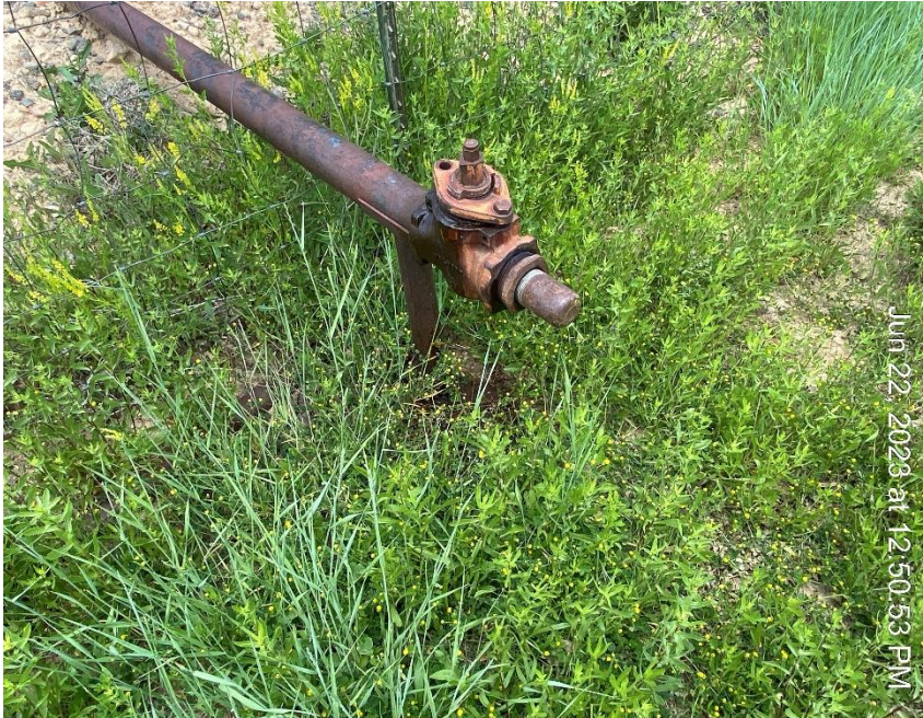
Leaky valve. Stained soil.
