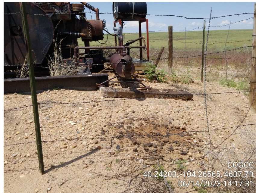
Photo 8 – Stained Soil at Exhaust
