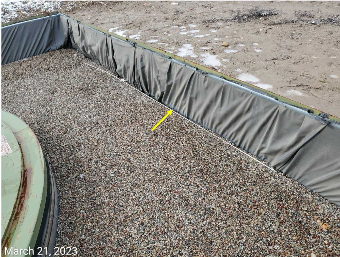
Photo 5: Photo shows unused pipe equipment remains improperly stored within containment BMP, on the Location
