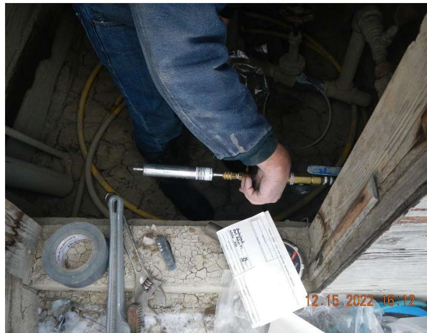
A gas sample was collected from the Bert Eaton (OWP) #1 during this inspection.
