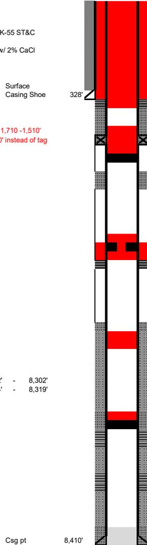
Perf TOC pump cmt inside and outside of csg (min 100 sx)
