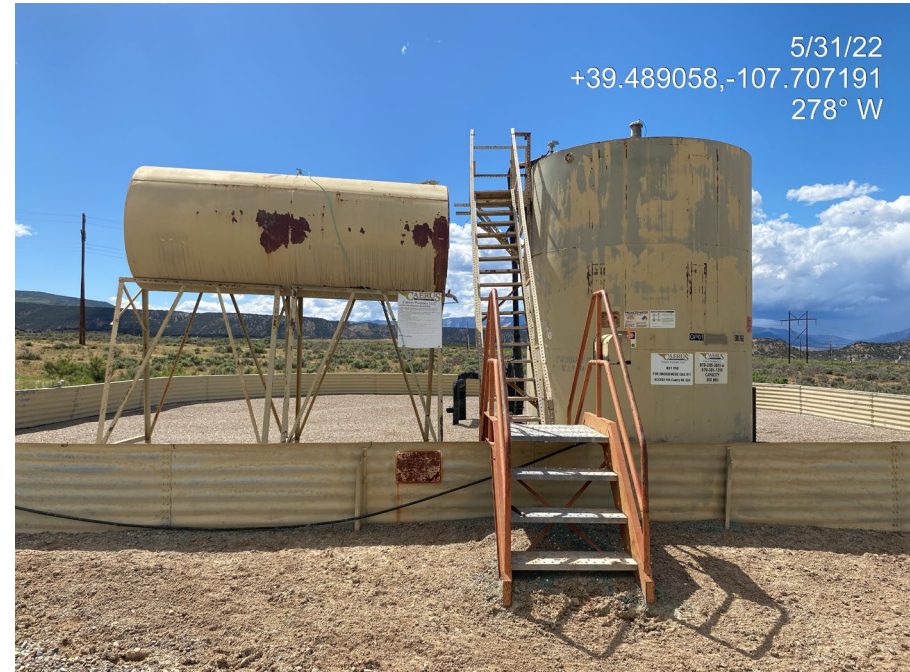
Photo 2. Photo taken from the tank battery at the north of the Location shows a lack of proper signage.
