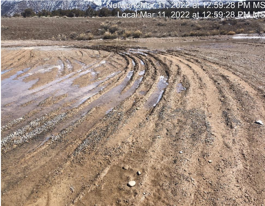
Photo #6153 Location lacks stabilization.
