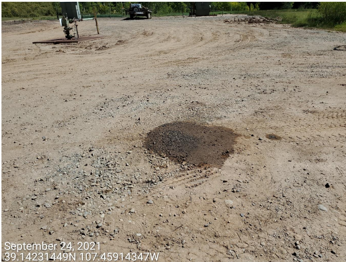
Photo 7: Photo shows stained soils observed to the southwest of the well.
