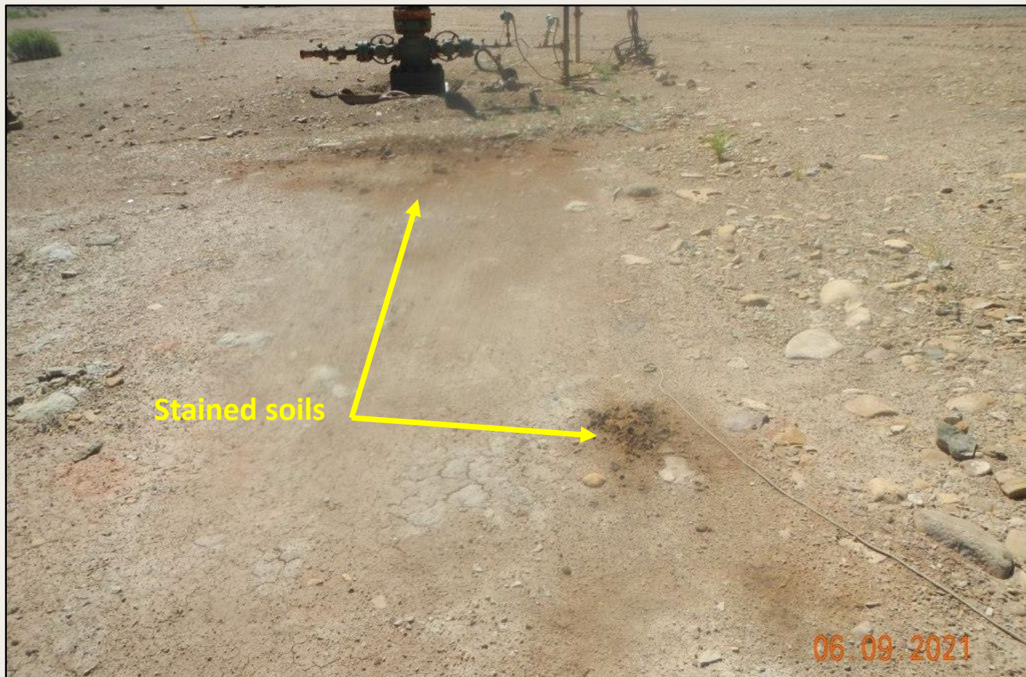
Photo 4. View of stained soils observed around the wellhead.
