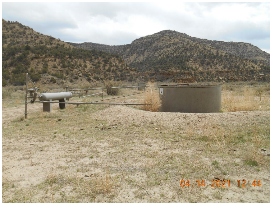
Produced Water tank and Separator.
