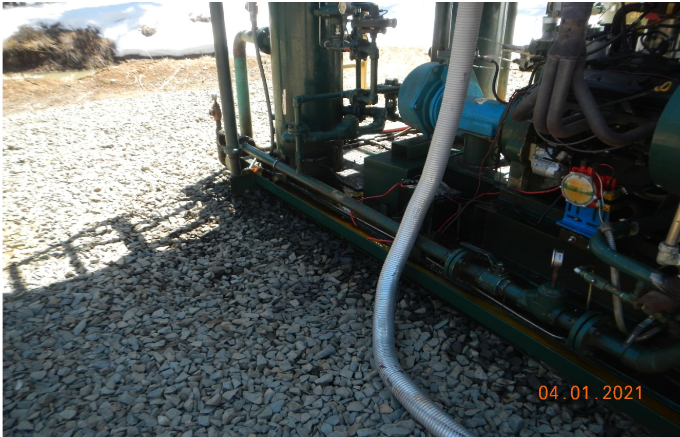
Photo 4. There is oil stained soil and oil in the engine skid which needs to be cleaned up.
