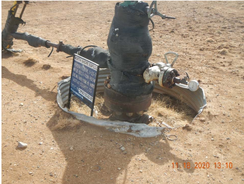
Photo 2. No bradenhead access apparent.
