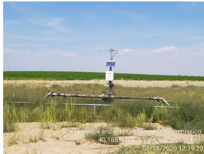
Photo 4 – Gas Meter – No current Calibration Card on Meter, Weeds
