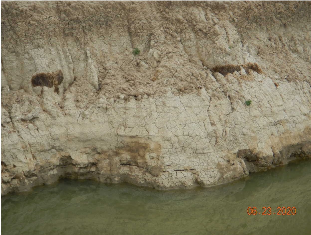
Photo # 7 – Pit ID 117639 subject of Spill ID 476164. Discontinuous oil stains in pit wall
