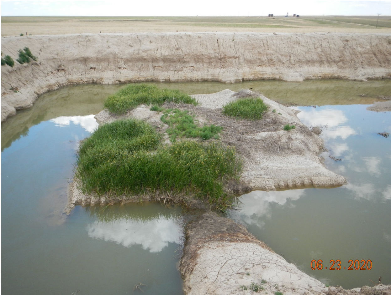
Photo # 9 – View east across Pit ID 117639 subject of Spill ID 476164. Discontinuous oil stained soil in eastern pit wall
