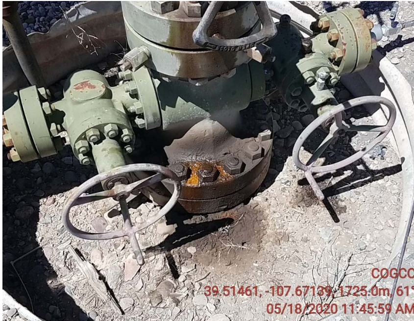
Master valve leaking
