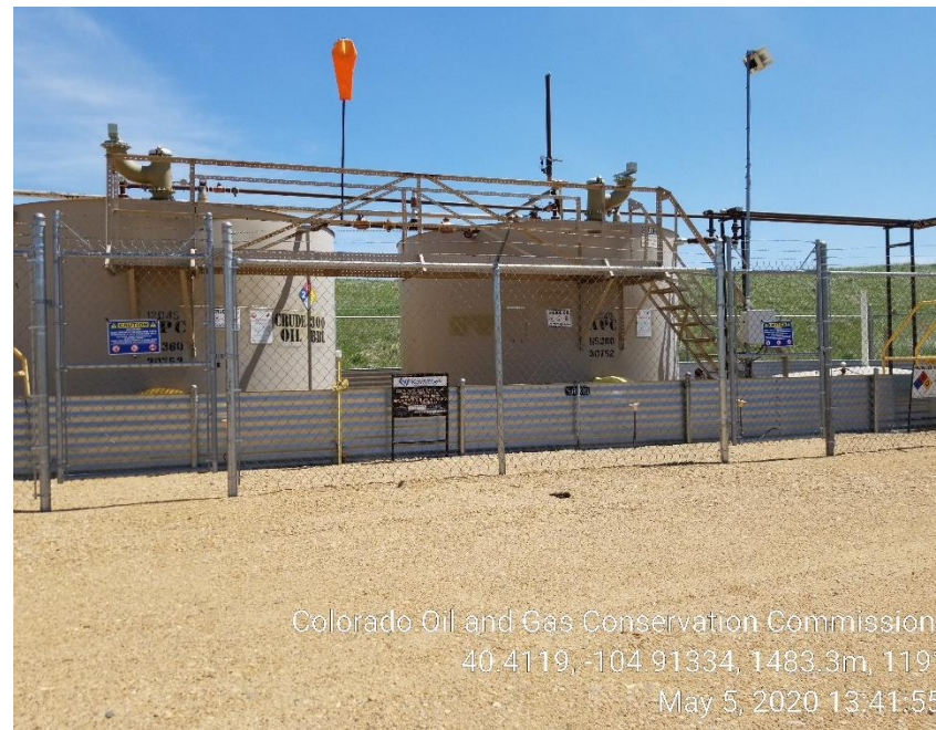
Photo 6: Tank Battery
