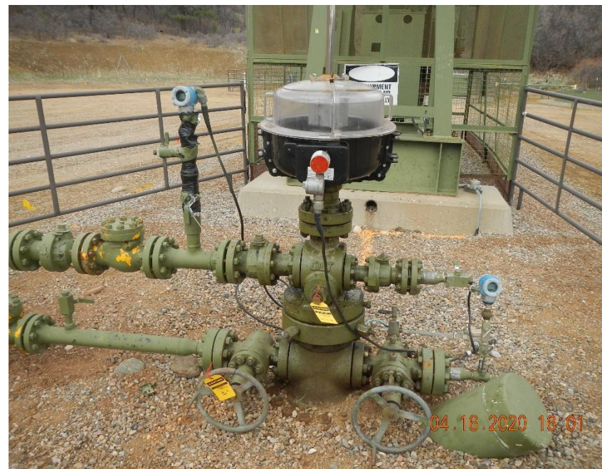
Containment device around stuffing box.
