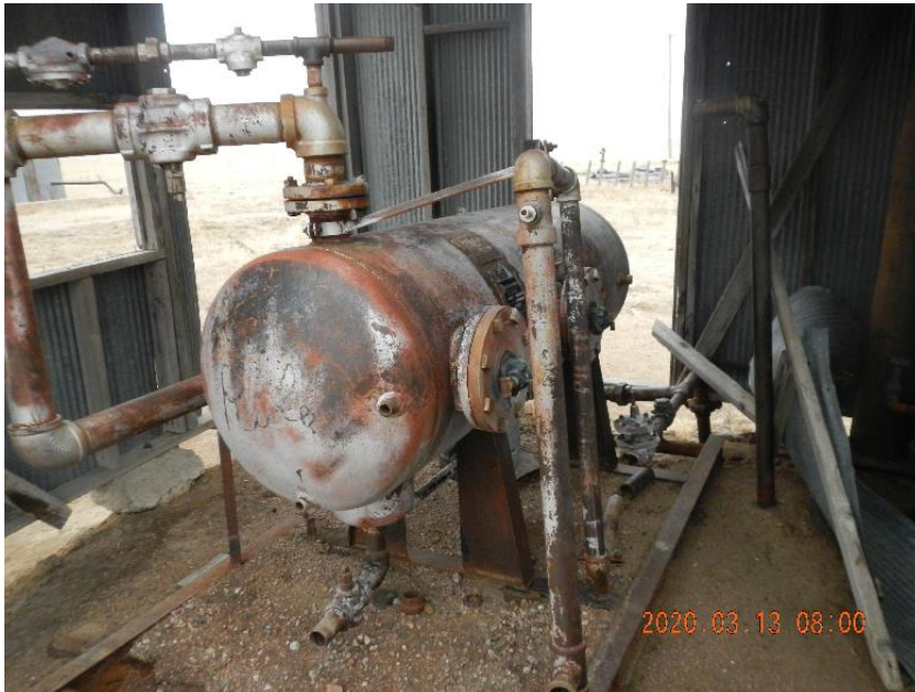
Photo 3: Separator and flow lines.
