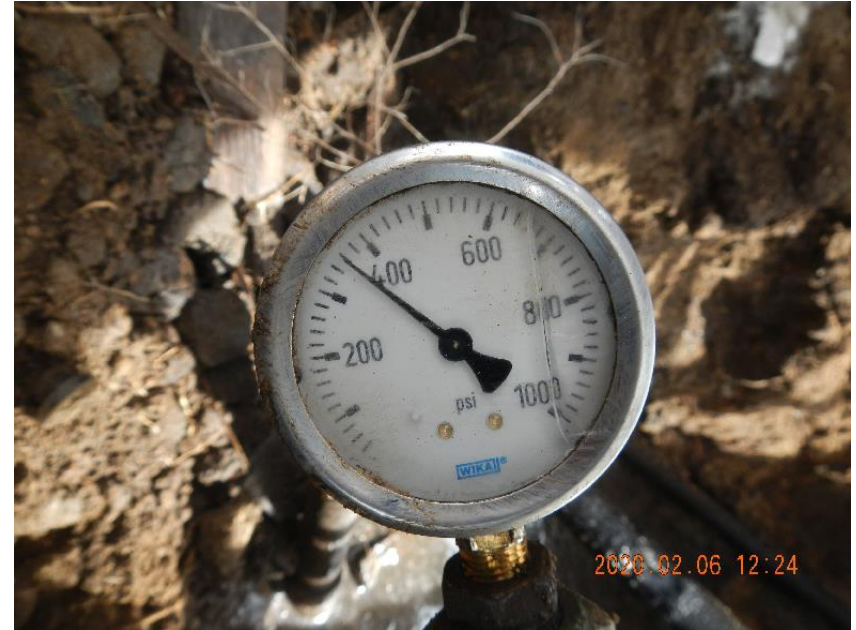
Photo 4: Completed pressure test.
