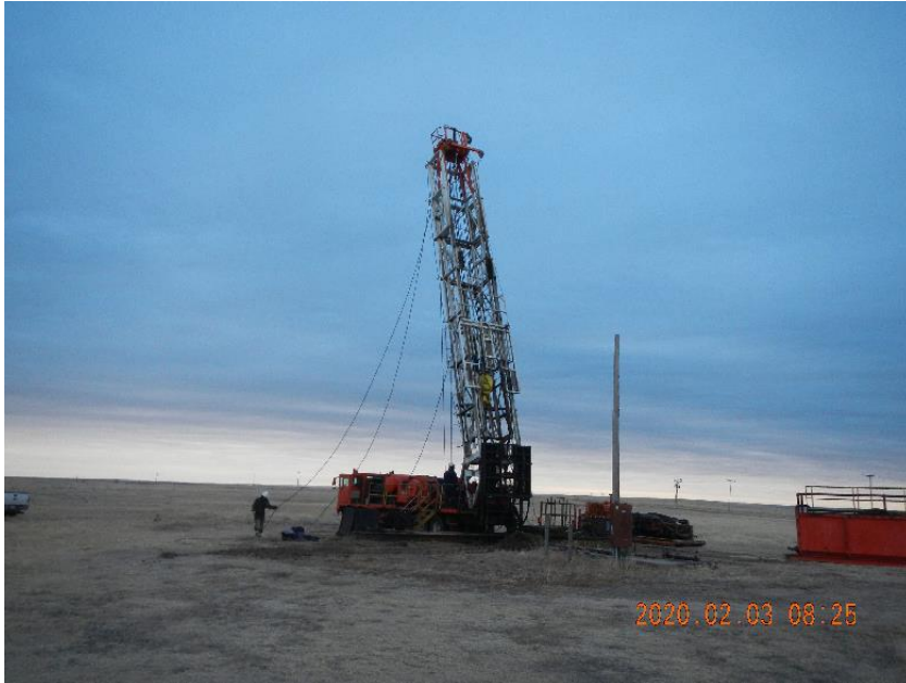
Photo 1: Rigging up on well.
