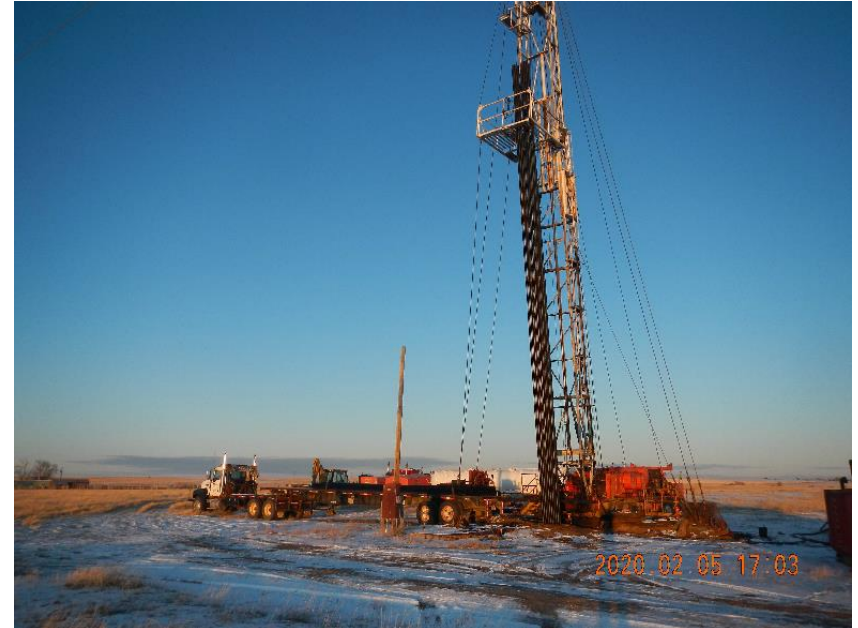
Photo 2: Tripping out tubing.
