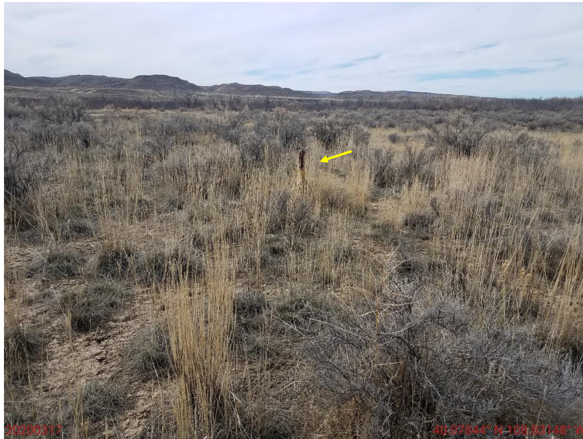
Photo 1: Photo taken from the well Location, facing west. Photo shows above grade well marker. Well marker is less than 4 feet AGL. An audible gas leak was detected coming from the well casing.
