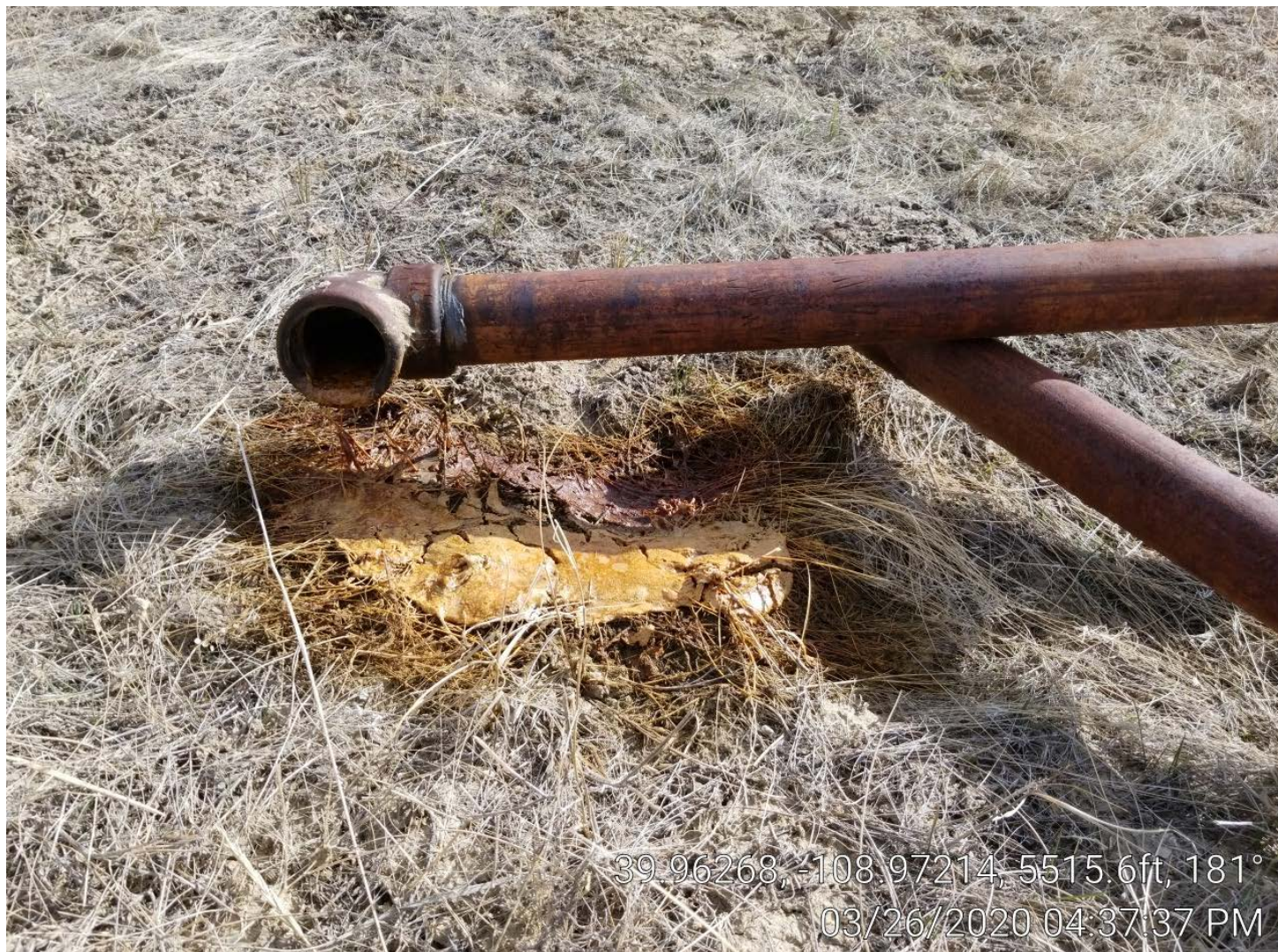
Photo 4. Hydrocarbon spill between separator & tank.
