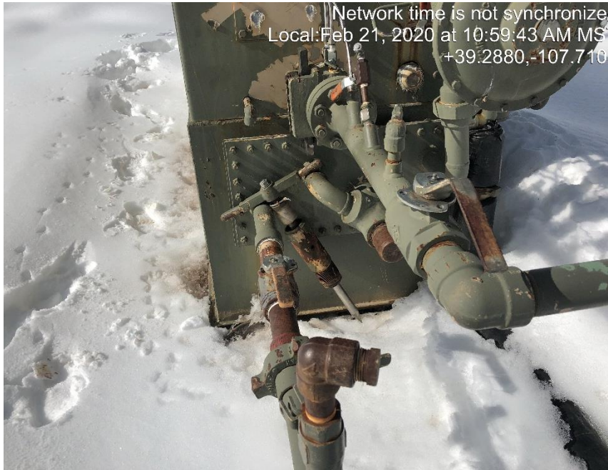
Photo #0622 Unused adjustable choke by separator.
