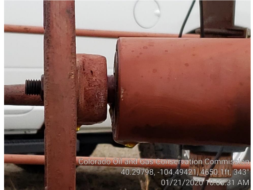
Photo #3 Leaking master valve
