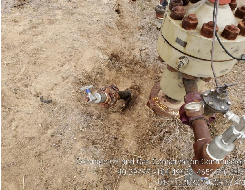
Photo #2 Stain soil from drip coming from master valve
