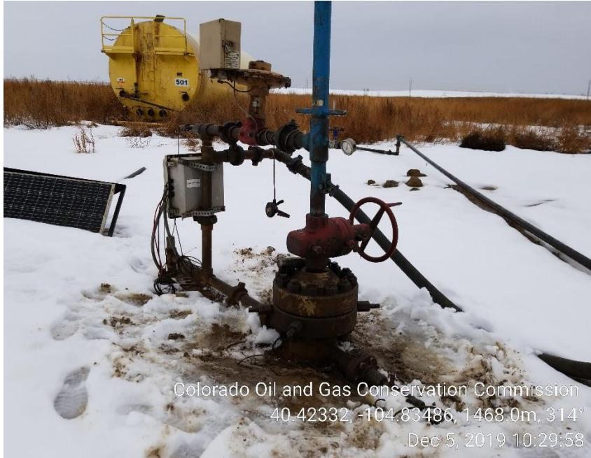
Photo 5: Wellhead; NO SIGNAGE
