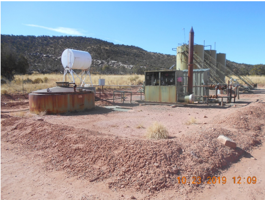
Separator, Meter housing and blowdown tank.
