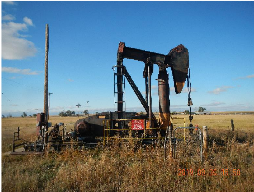
Photo 1: Pumping unit and power pole.
