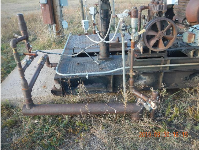
Photo 9: View of risers and flow lines at back of pumping unit.
