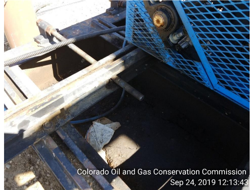
Photo 4 Stained soil under PU motor
