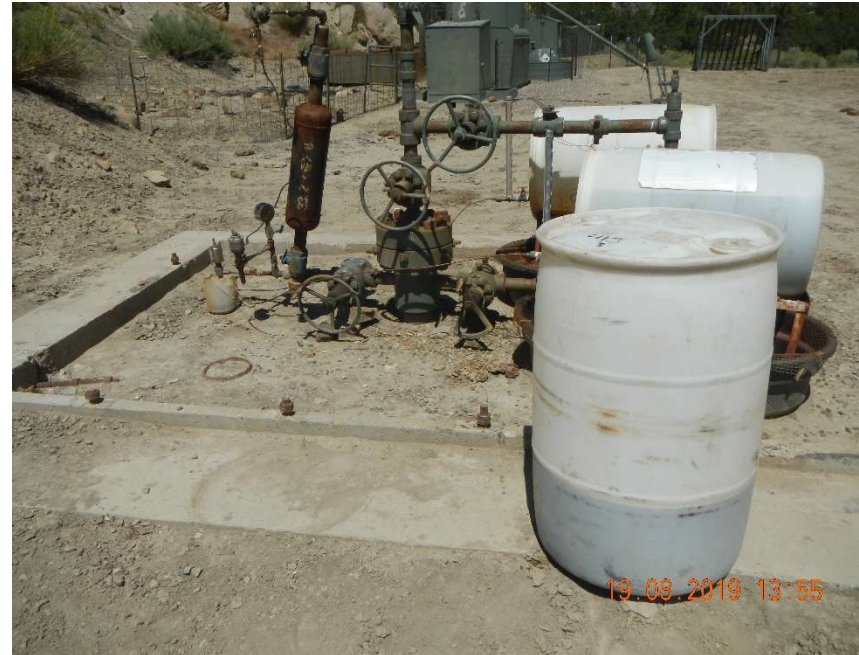
Photo #8 - Inadequate berms around day tank south of well.
