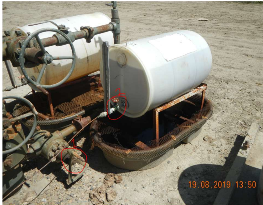
Photo #11 – View of the two active leak locations.
