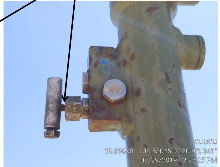
Photo 3. Well head gas leak.
