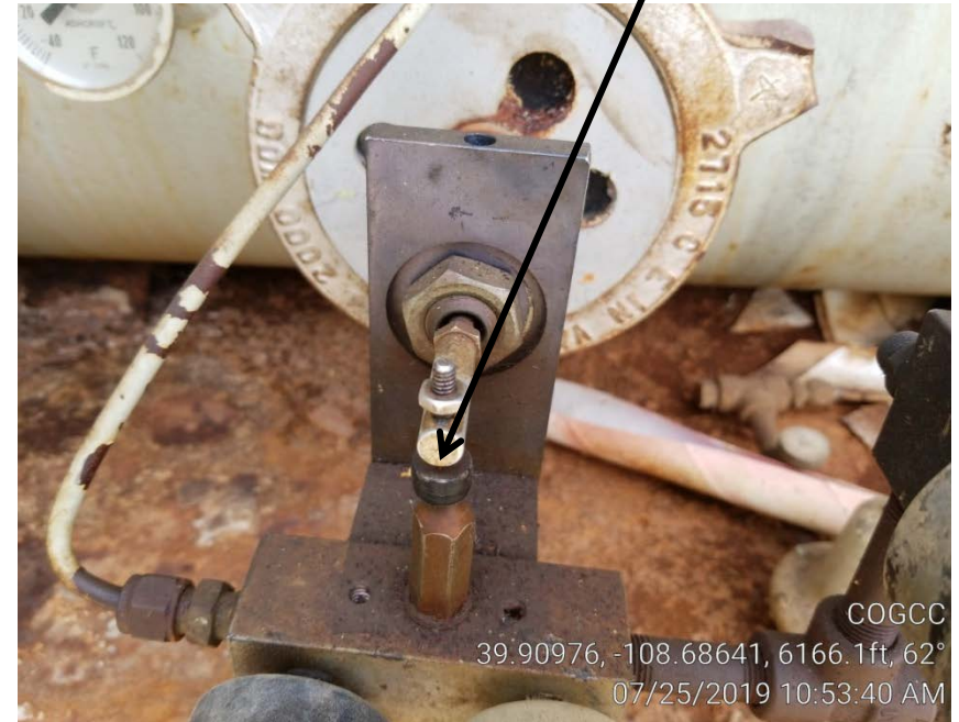
Photo 5. Separator gas leak.
