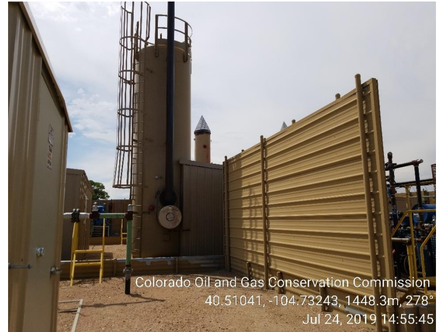
Photo 8: (North) Heater treater with supplies/trash
