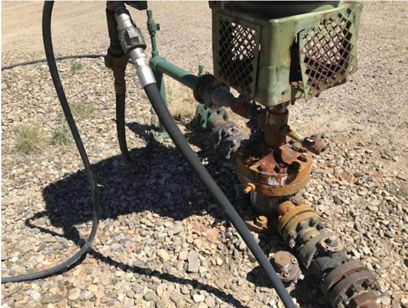
PHOTO 3: THE IMPACTED SOIL AROUND THE WELL HEAD WAS REMOVED AND THE PACKINGS WERE REPLACED TO STOP THE WATER LEAK.
