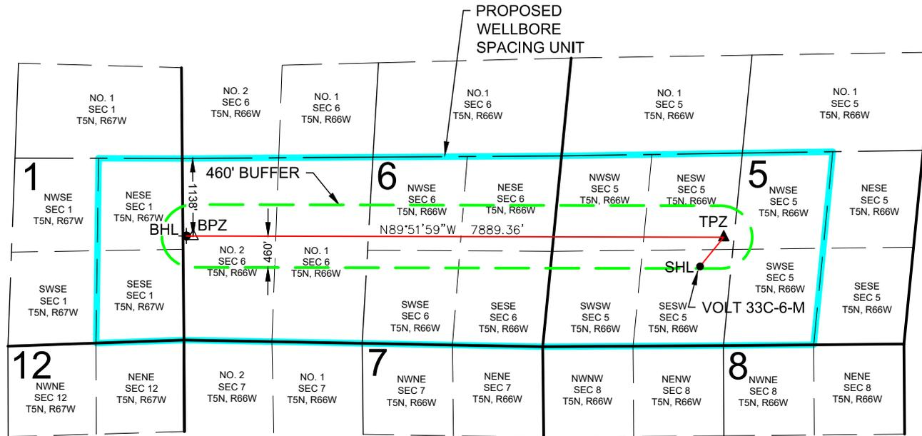
**VOLT 33C-6-M WELL TO BE LOCATED 1165' FSL AND 2182' FWL, SEC 5, T5N, R66W**
