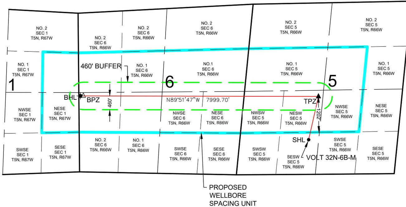
**VOLT 32N-6B-M WELL TO BE LOCATED 1163' FSL AND 2301' FWL, SEC 5, T5N, R66W**
