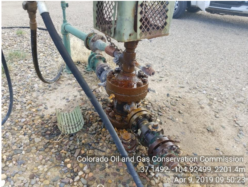
Photo 3 Stained soil around WH and packing leaking on well head.
