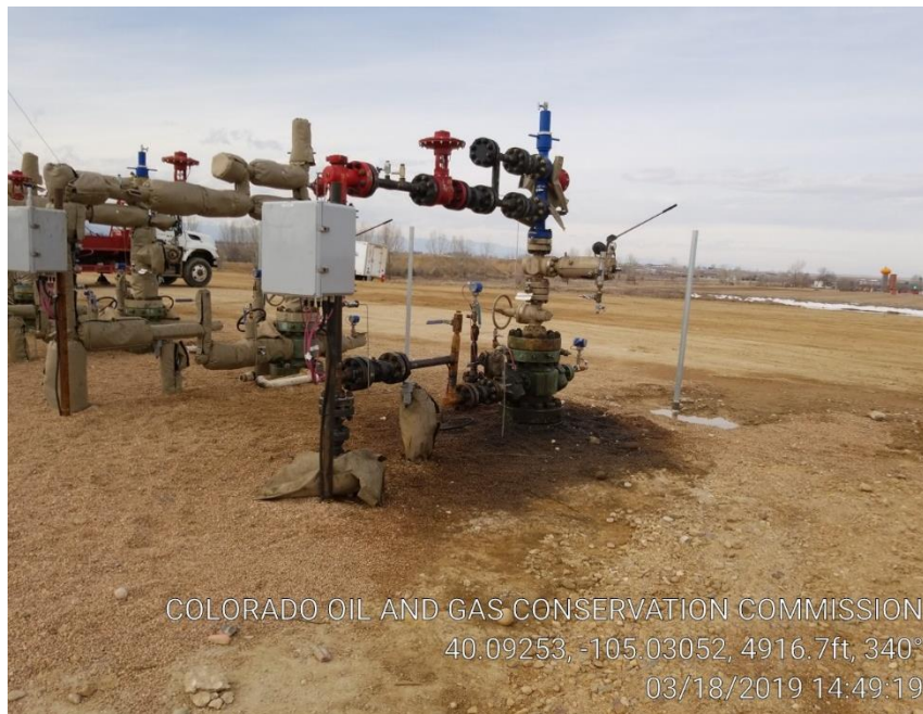
Pic 1, stained soil around wellhead from workover.
