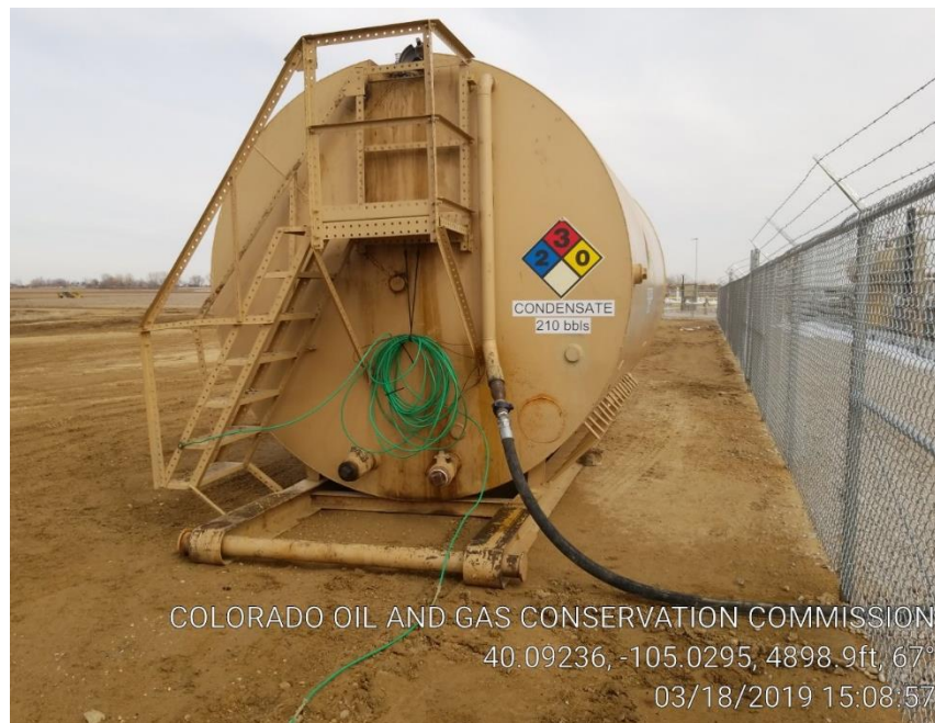
Pic 25. Temporary tank being used to collect crude oil.
