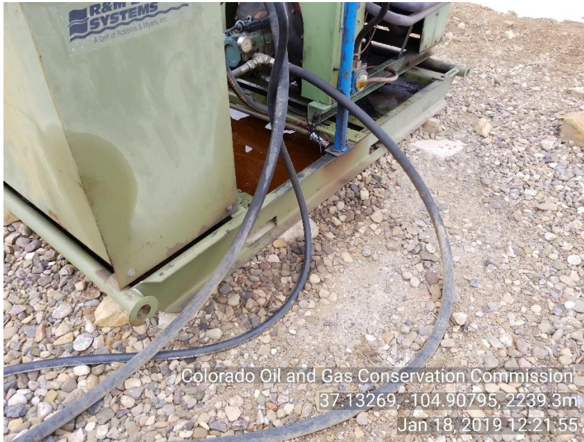
Photo 3 stained soil around HYD motor skid
