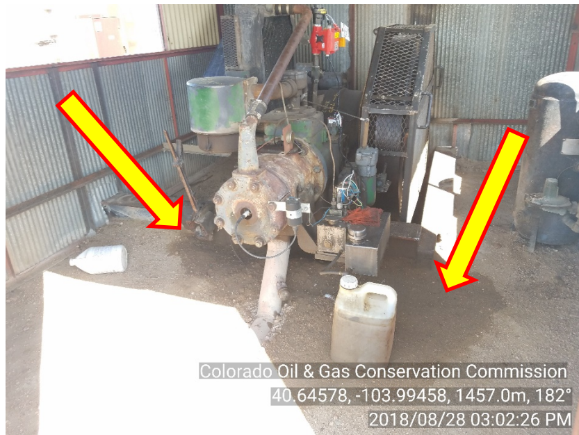
Photo #5 Malo 9-20 Pump jack engine house Stained soil around engine
