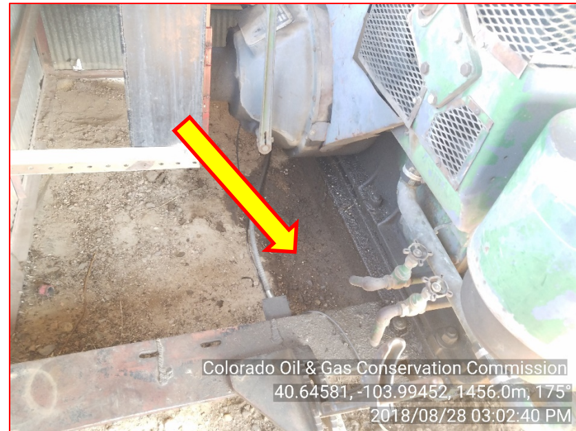
Photo #6 Malo 9-20 Pump jack engine house Stained soil around engine base
