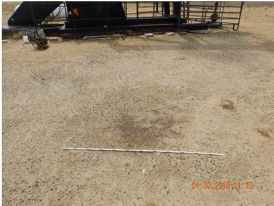
Photo 19: Photo taken from the northwest side of the well. Photo shows stained soil. 6 foot measuring stick for reference.
