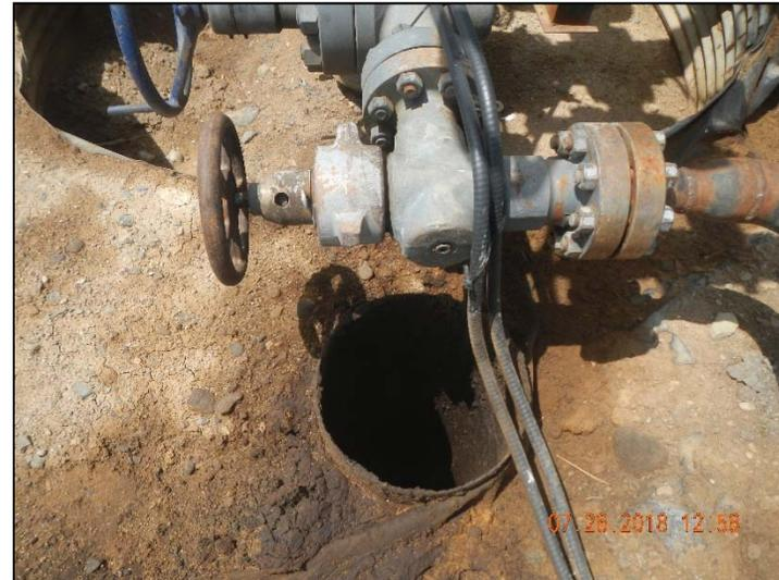
**Photo 2. Rathole open at wellhead.**
