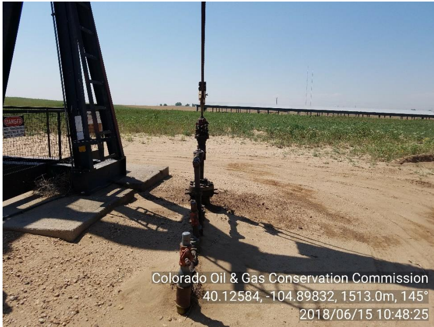
Photo 3. Stained soil around wellhead
