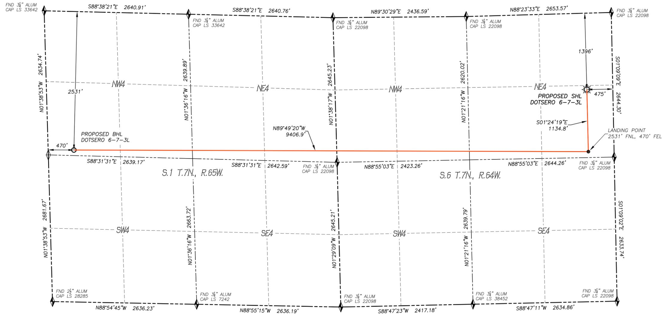
IN ACCORDANCE WITH A REQUEST FROM CONFLUENCE RESOURCES, DALEY LAND SURVEYING, INC. HAS DETERMINED THE SURFACE LOCATION OF THE DOTSERO 6-7-3L WELL TO BE 1396' FNL, 475' FEL, AS MEASURED AT NINETY (90) DEGREES FROM THE SECTION LINES OF SECTION 6, TOWNSHIP 7 NORTH, RANGE 64 WEST, AND THE BOTTOM HOLE LOCATION TO BE 2531' FNL, 470' FWL, AS MEASURED AT NINETY (90) DEGREES FROM THE SECTION LINES OF SECTION 1, TOWNSHIP 7 NORTH, RANGE 65 WEST, OF THE 6TH PRINCIPAL MERIDIAN, WELD COUNTY, COLORADO.
