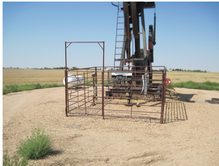
wellhead and pump jack
