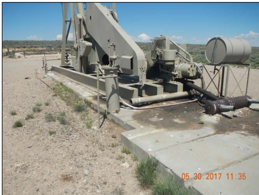
Photo 4. Flowlines to separator and motor for pump jack.
