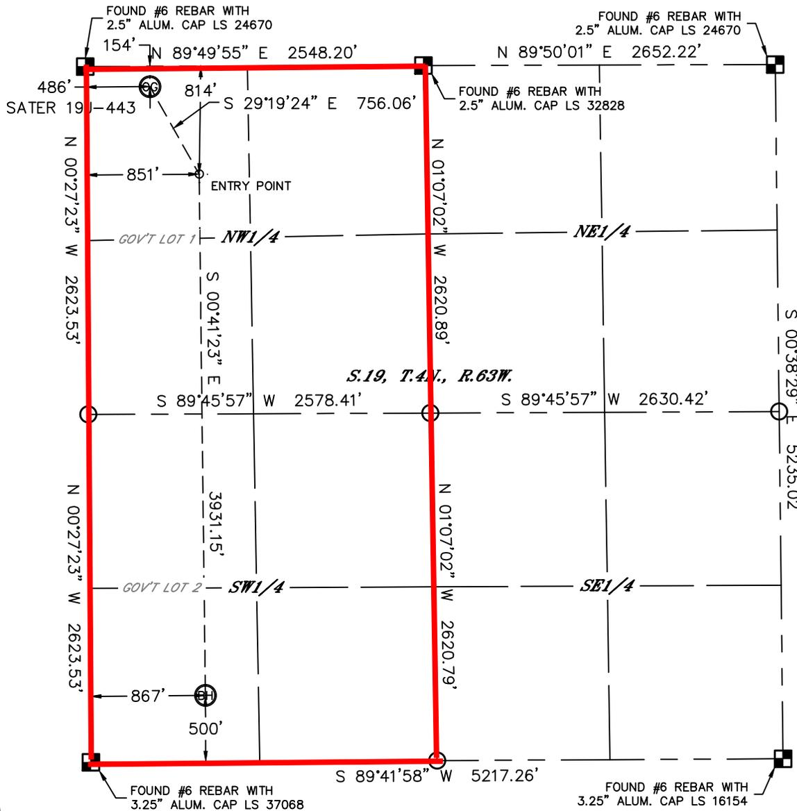
In accordance with a request from Mac Neumann with PDC ENERGY Lat40°, Inc. has determined the surface location of the SATER 19J-443 to be 154' from the NORTH line and 486' from the WEST line and the bottom hole to be 500' from the SOUTH line and 867' from the WEST line as measured at right angles from the section lines of Section 19, Township 4 North, Range 63 West of the Sixth Principal Meridian, County of Weld, State of Colorado.
