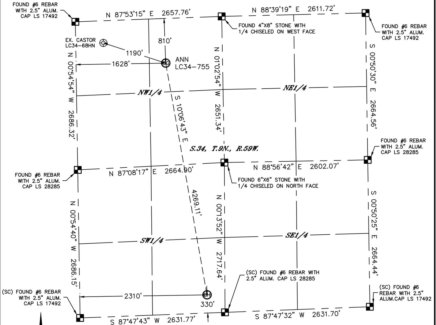
In accordance with a request from Brian James with Noble Energy Inc. Lat40°, Inc. has determined the surface location of the ANN LC34-755 to be 810' from the NORTH line and 1628' from the WEST line and the bottom hole to be 330' from the SOUTH line and 2310' from the WEST line as measured at right angles from the section lines of Section 34, Township 9 North, Range 59 West of the Sixth Principal Meridian, County of Weld, State of Colorado.
