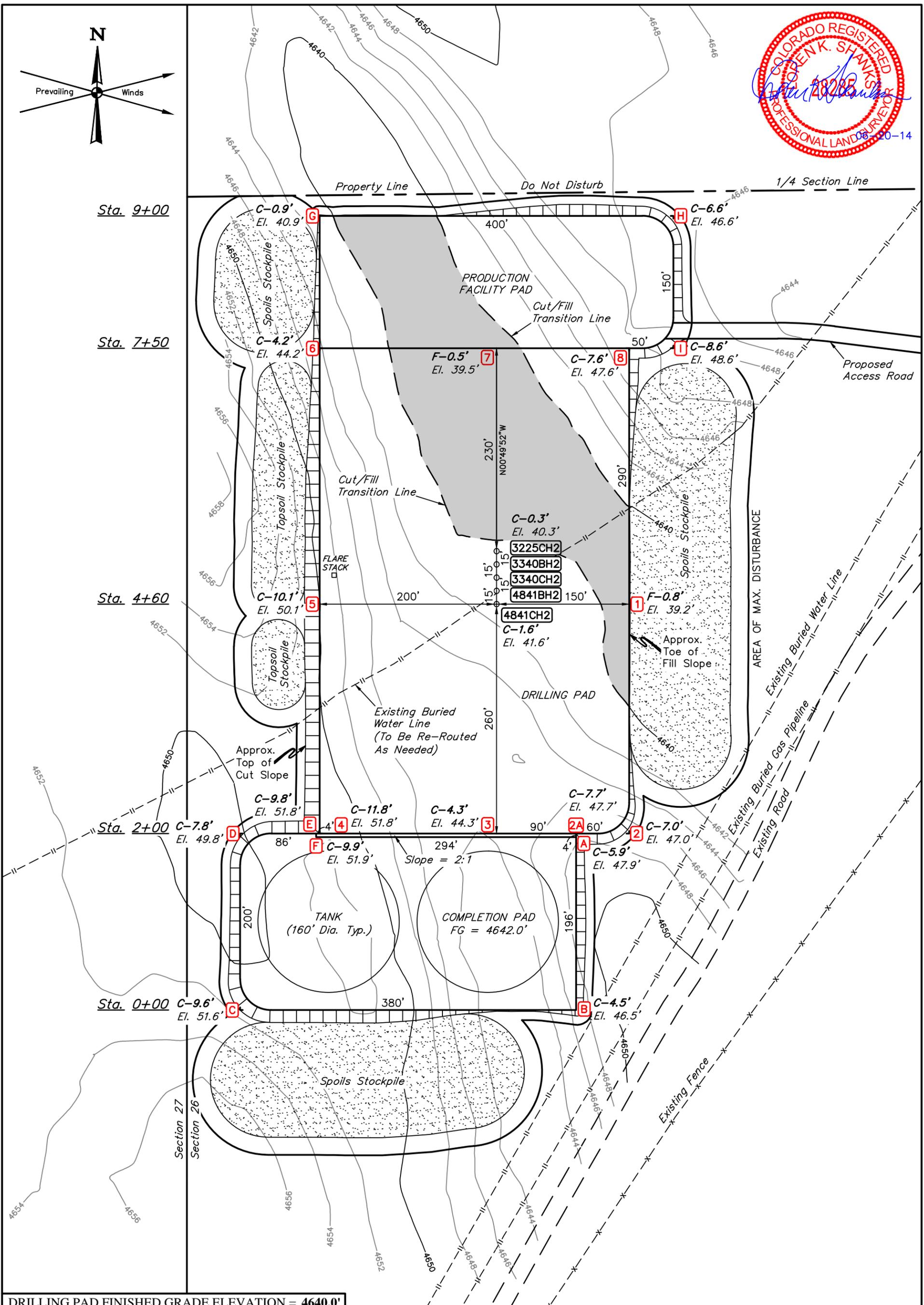
**DRILLING PAD FINISHED GRADE ELEVATION = 4640.0'**
